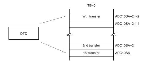
The internal address pointer is initially equal to ADC10SA and the internal transfer counter is initially equal to 'n'. The internal pointer and counter are not visible to software. The DTC transfers the word-value of ADC10MEM to the address pointer ADC10SA. After each DTC transfer, the internal address pointer is incremented by two and the internal transfer counter is decremented by one.
